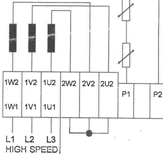
P1, P2 = PTC THERMISTORS (MAXIMUM VOLTAGE 2,5 VDC)
