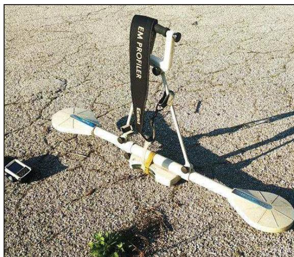
Figura 2.2 – Elettromagnetometro Profiler EMP-400
