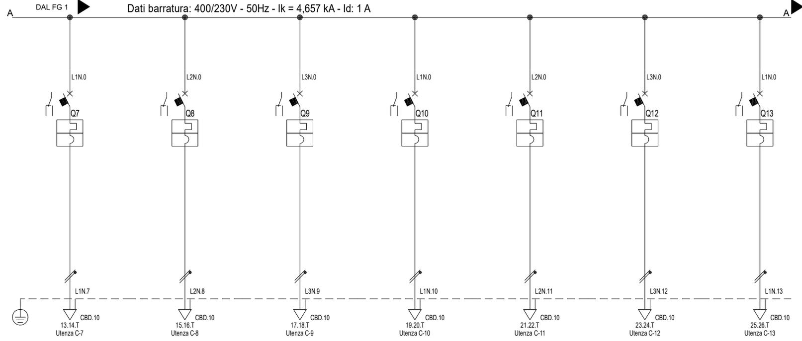
Dati barratura: 400/230V - 50Hz - I<sub>k</sub> = 4,657 kA - I<sub>d</sub>: 1 A
