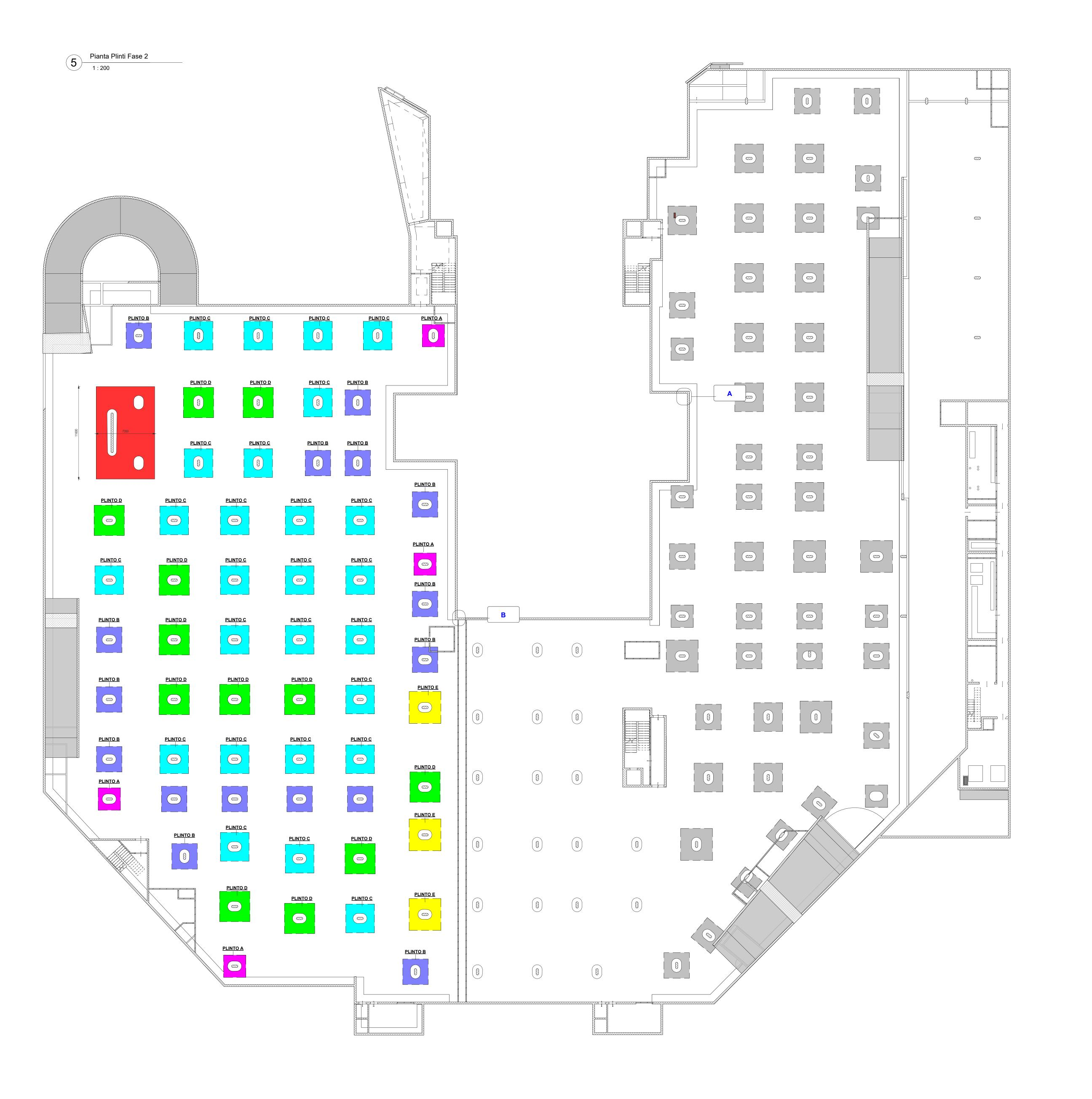
**LEGENDA**: PLINTO A 2.8x2.8x1.5m PLINTO B 3.2x3.2x1.5m PLINTO C 3.6x3.6x1.5m PLINTO D 3.8x3.8x1.5m PLINTO E 4x4x1.7 PLINTO F 7.35x11.6x1.5m
