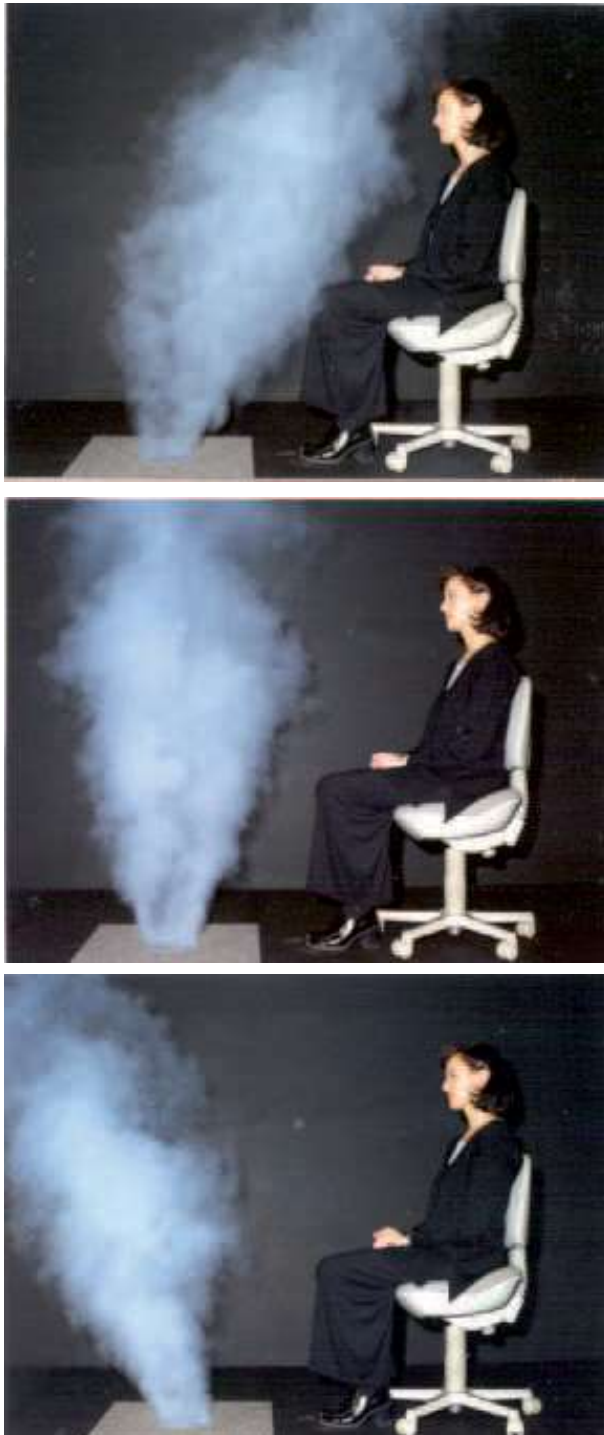
Figure 3: Jet pattern for different settings, shown for size DN 200
