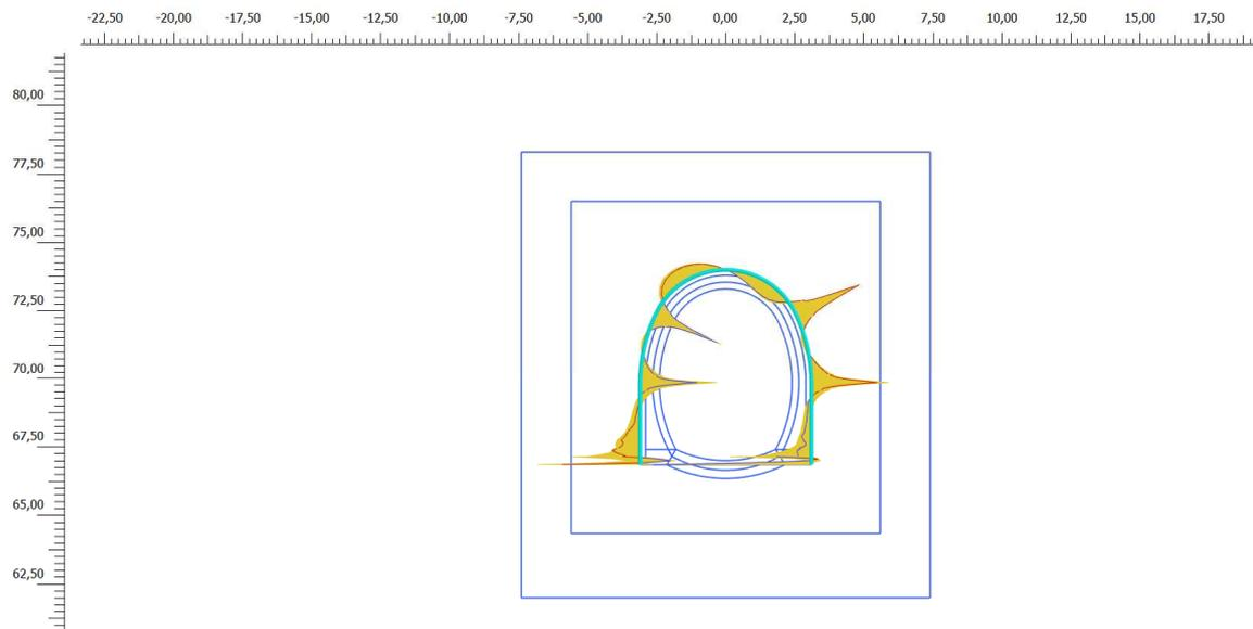
Envelope of Shear forces Q (scaled up 0,200 times)
